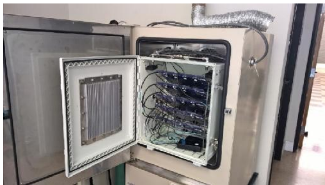
Figure 1: Characterization Test System Example – Sealed box inside of environmental chamber capable of holding a large number of units under test.
