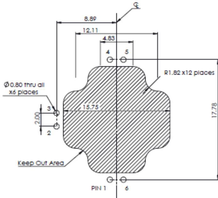
Dimensions are in millimeters
